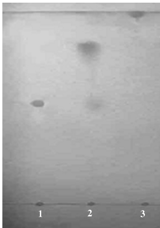
Fig. 2. TLC result from fermentation of Penicillium sp. Li-3 (Note: (1) GL standard; (2) fermentation form Penicillium sp. Li-3; (3) glycyrrhetic acid standard). while the molecular weight of GAMG was 648. The difference between them may be caused by the lost of hydrogen ion during ionization. From Fig. 3, it could be clearly known that the main metabolism production of this strain using GL as substrate was GAMG.
